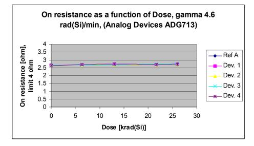
Figure 4 On resistance as a function of Dose, gamma 4.6 rad(Si)/min.
