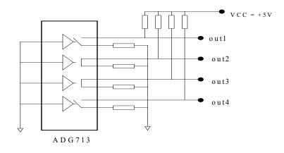
Figure 1 Simplified schematic diagram of the ADG713 irradiation biasing board.
