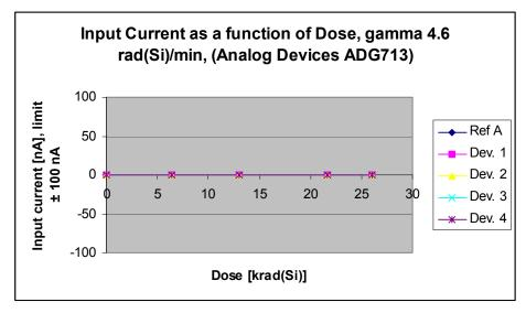
Figure 2 Input current as a function of Dose, gamma 4.6 rad(Si)/min.
