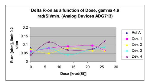
Figure 3 Delta R-on as a function of Dose, gamma 4.6 rad(Si)/min.
