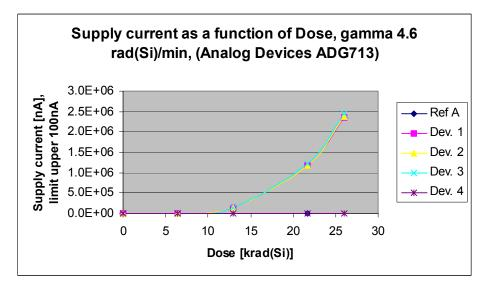
Figure 5 Supply current as a function of Dose, gamma 4.6 rad(Si)/min.
