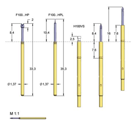
This series was developed for difficult contacting conditions such as lead free soldered or strongly contaminated pads or oxidized boards. Probes of this series allow penetrating sticky layers reliably with a low vulnerability to contaminations of the tips. All this leads to a high contact reliability and a long life time of these probes. Further information about the receptacles see extra section for receptacle H100.
