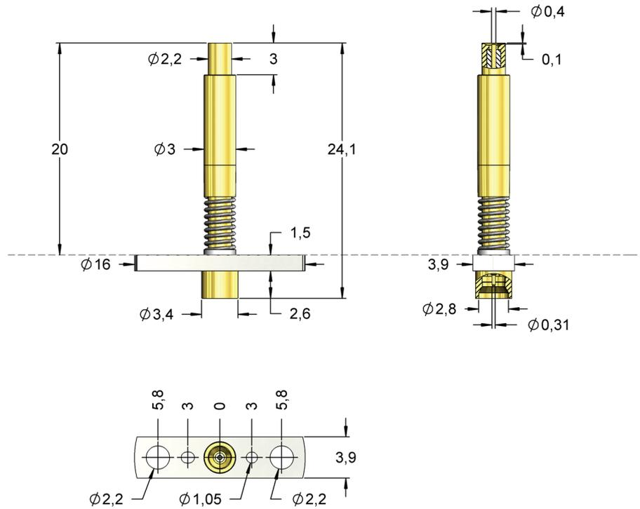
The probe can be mounted using the flange.
