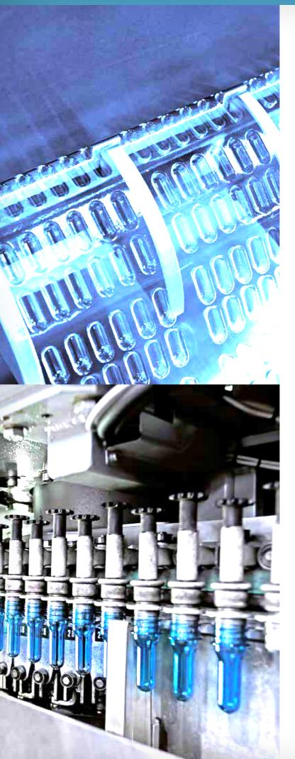
Example of blister packaging: a uniform seal pattern on blister packaging requires high precision in insulating components with respect to plane parallelism. This is compounded by even larger tool dimensions with higher numbers of cavities.
