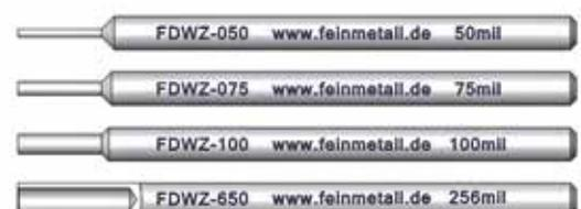
For inserting the probe into the receptacle tool FDWZ is helpful. After the probe is pushed into the receptacle and stopped by the pressure marks, the probe is driven into the receptacle with the FDWZ tool. The tool is made of a synthetic material to avoid any damaging of the plunger tips.
