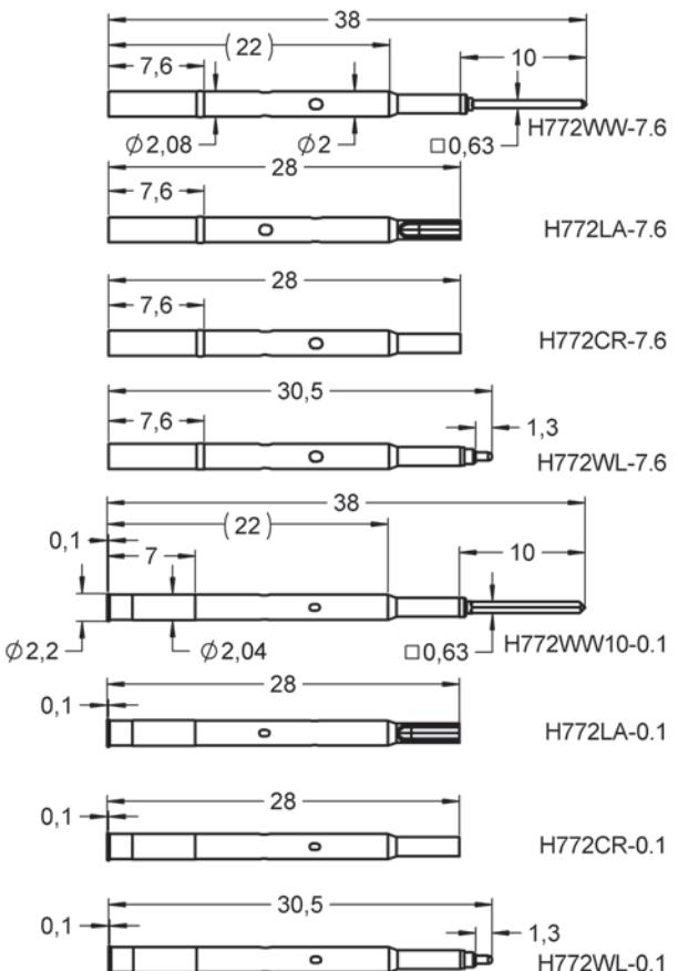
The insertion depth 22 mm and outer diameter are the same for all receptacles shown above. Different dimensions are listed.
