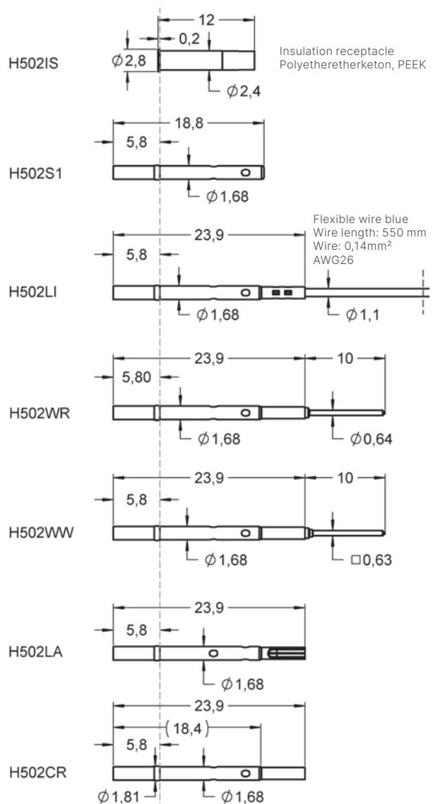
The insertion depth 18.4 mm and outer diameter are the same for all receptacles shown above. Different dimensions are listed.
