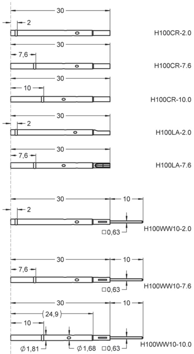
The insertion depth 24.9 mm and outer diameter are the same for all receptacles shown above. Different dimensions are listed.
