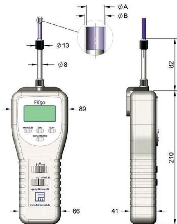
Operating manual available on request. Further rigid measuring sleeves with different diameters and fixed projection height are available on the homepage.
