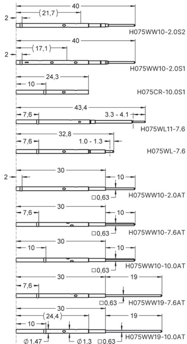
The insertion depth 24.4 mm and outer diameter are the same for all receptacles shown above. Different dimensions are listed.
