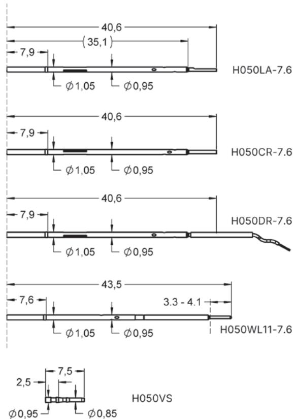
The insertion depth 35.1 mm and outer diameter are the same for all receptacles shown above. Different dimensions are listed.
