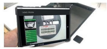
With a tablet device and a mobile version of the labels software, you are able to handle each kind of packaging. Bulky and heavy material excludes handling at the incoming goods scanner. That's why MODI offers the ability to capture product labels with a mobile solution.
