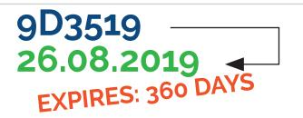
The manufacturers of the components encrypt their production date on the reel. If you want to use this date for calculation, for example, the durability of the component, you must convert it into a "real" date. The label software now offers this feature.
