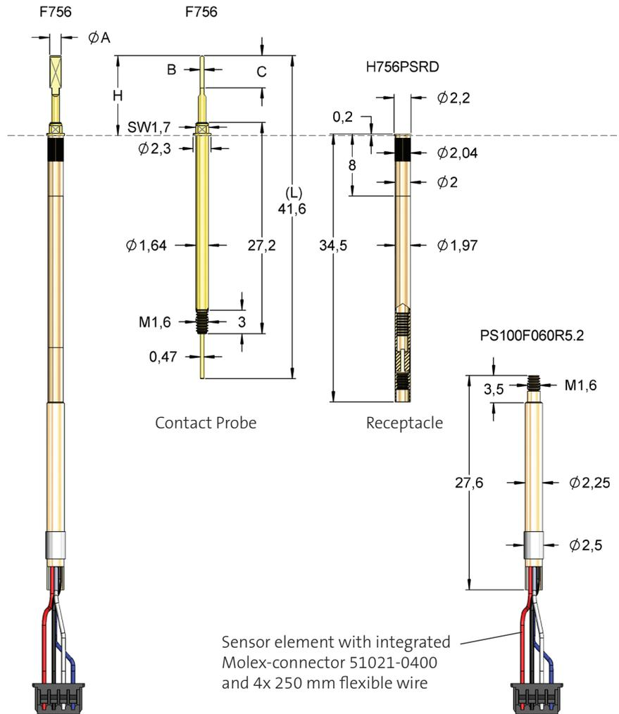
The position sensor system consists of a twist proof threaded probe F756..., a receptacle H756PS and a sensor element PS100.... These three elements are mounted into a fixture plate. The position sensor is screwed at the receptacle from backwards after the receptacle is mounted.
