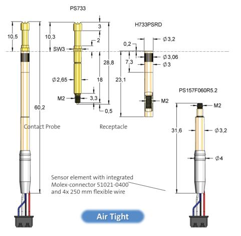
The position sensor system PS733 can be used in vacuum fixtures or modules (max. leakage rate <0,5 cm<sup>3</sup>/min at 0,7bar). It consists of a special spring contact probe PS733..., a receptacle H733PSRD and a sensor element PS157.... These three elements are mounted into a fixture plate. The position sensor is screwed at the receptacle from backwards after the receptacle is mounted.
