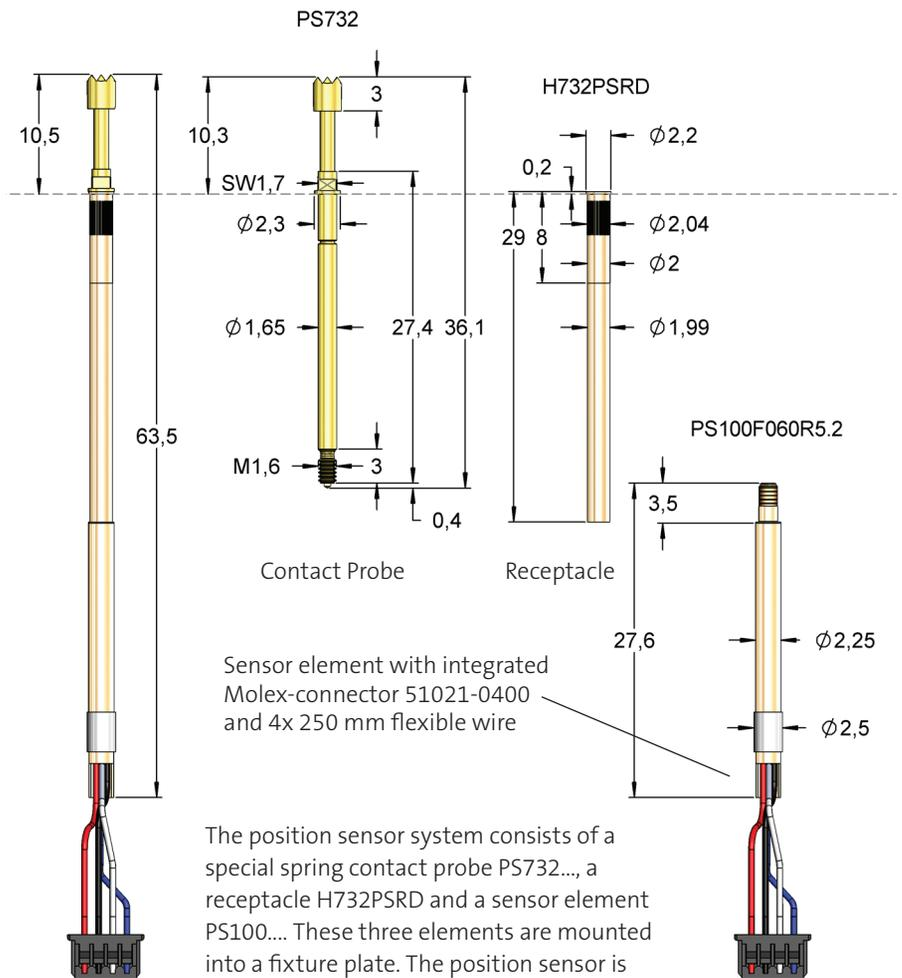
The position sensor system consists of a special spring contact probe PS732..., a receptacle H732PSRD and a sensor element PS100.... These three elements are mounted into a fixture plate. The position sensor is screwed at the receptacle from backwards after the receptacle is mounted.
