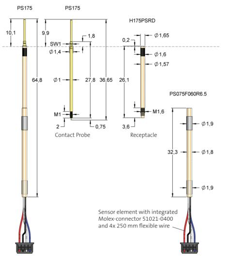
The position sensor system consists of a special spring contact probe PS175..., a receptacle H175PSRD and a sensor element PS075.... These three elements are mounted into a fixture plate. The position sensor is screwed at the receptacle from backwards after the receptacle is mounted.
