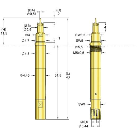
For contacting PCBs coaxial closed.
