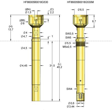
For contacting Reverse SMA-Female connectors.
