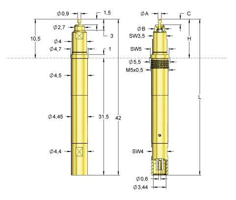
For contacting mini SMP-Female connectors.
