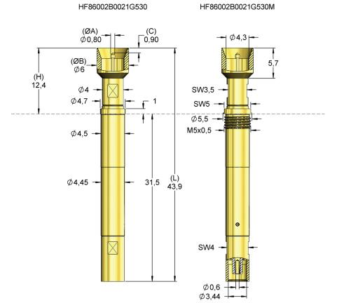
For contacting DIN 1,0/2,3-Female connectors.
