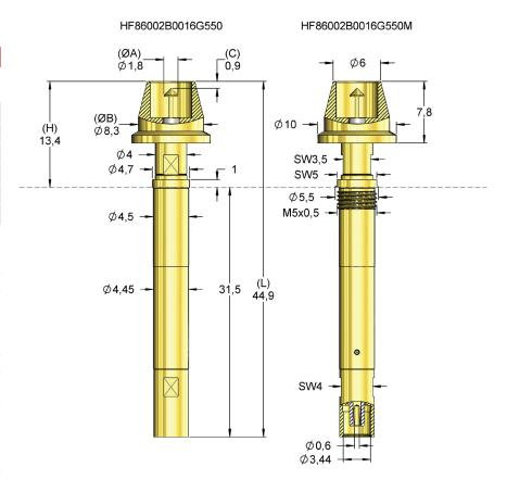
For contacting BNC-Female connectors.
