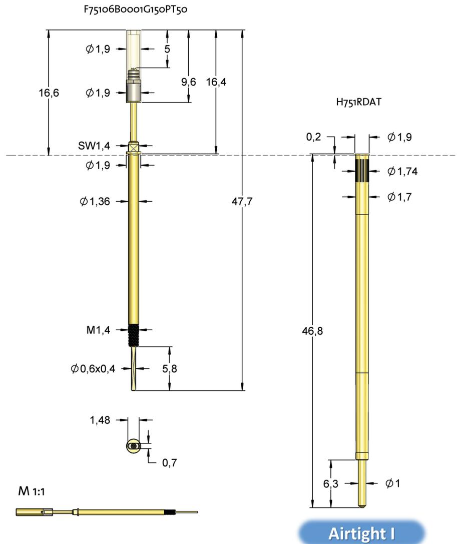
Further details of version **F75106B0001G150PT50** (slot 0,7 x 1,48 mm) with twist proof insulation cap see applications on page 83.
