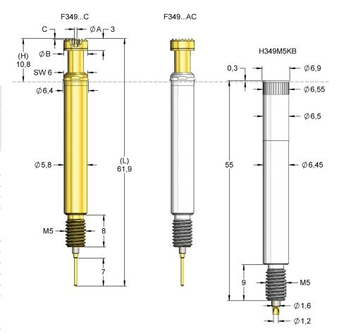
The new high current Kelvin probe F349C allows 4-wire measurements with currents up to 100 A even at smaller power components with centers down to 300 mil. The robust design allows applications even at rough production conditions. The F349C is mounted into the receptacle H349M5KB. The circular contact is connected by the M5 thread of the receptacle. It can be mounted with a counternut to a cable eye. The internal contact at the receptacle needs to be soldered.
