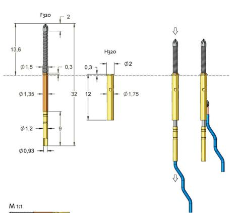
The continuous plunger guarantees a low internal resistance and allows applications with high currents. The connection of the plunger should be realized by a flexible wire with sufficient space for the movement. The wire can also be soldered directly to the receptacle. However, this leads to a lower electrical performance.
