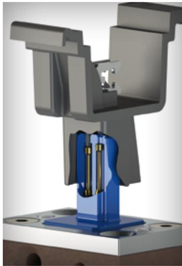
Not OK contact pin is bent
