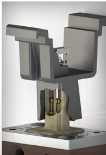
Not OK contact pins = abrasion/dirt
