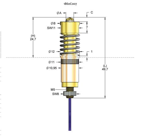
Der 1860C007 adapts to an up to 1,5 degree inclined surface. The M5 thread can be mounted with a counternut to a cable eye.
